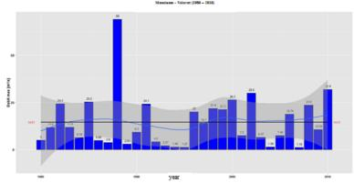
Fig. 6.33 The annual maximum debits at the Manoleasa hydrometric station, Volovăţ River
